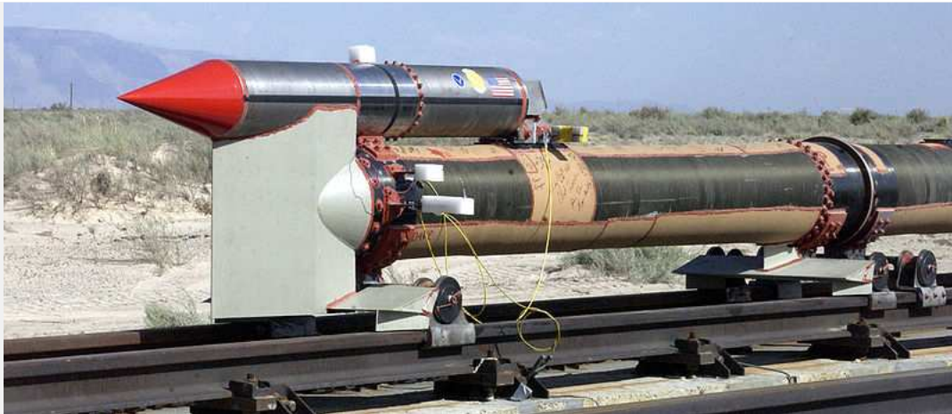
Rail Track Rocket Sled - Penta Rail Supersonic Track at Terminal Ballistics Research Laboratory
