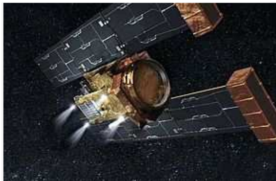
Artist's rendering of Stardust-NExT performing a burn-to-depletion during the decommissioning of the spacecraft.
